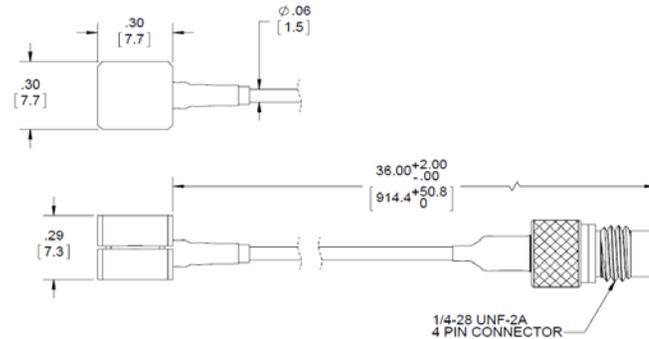
Units on the line drawing are in inches, units in brackets are in millimeters. Refer to 127-3133B4 for more information.
