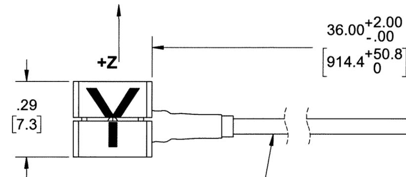
7 CABLE, 4-CONDUCTOR, SHIELDED, WHITE JACKET. SEE TABLE FOR SPECIFICATIONS
