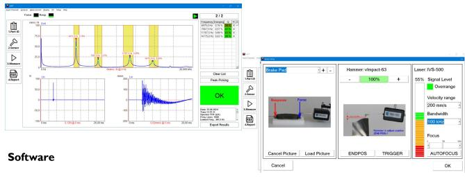
The software receives the Meta Data for the test object, starts the measurement and sends the "Fail/OK" information to a PLC or a digital output.
