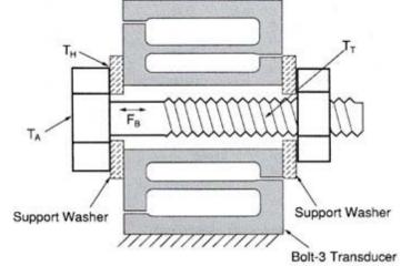
These rugged transducers are manufactured with high-strength aluminum shells (alloy 7075-T6) and either aluminum or 17-4 PH stainless steel sensing elements. A durable anodized finish protects the aluminum from corrosion while elastometric Oring seals protect the strain gages and wiring.
