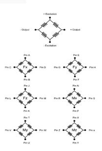
Bridge Fz; Mz = 700 ohms Bridges Fx; Fy = 350 ohms Connector Type: Souriau 851-02E16-26P50-44
