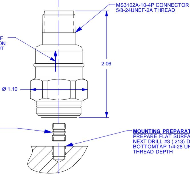
ARROW INDICATES SENSE OF DIRECTION OF ACCELERATION FOR POSITIVE GOING OUTPUT SIGNAL
