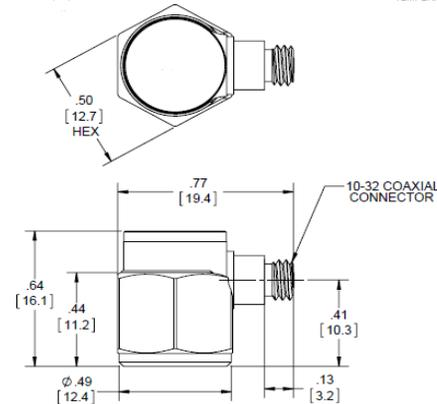
Units on the line drawing are in inches, units in brackets are in millimeters. Refer to 127-3055D for more information.
