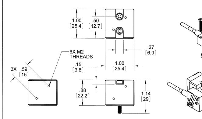
M2X.4 X12MM MOUNTING SCREW (SUPPLIED WITH 7521A)
