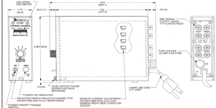
Units on the line drawing are in inches, units in brackets are in millimeters. Refer to 127-4114B1 for more information.
